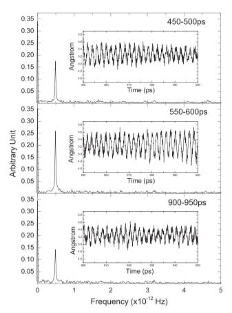
**Fig. 2.** Frequency-domain analysis of the radial movements of a carbon atom located in the center portion of the outer nanotube before (upper panel), during (middle panel), and after (lower panel) the hibernation period of the intertube axial oscillation. Initial extrusion s = 27.5 Å, and  $T_i = 300$  K. Insets: corresponding time-domain pictures for the radial movements of the same carbon atom.
