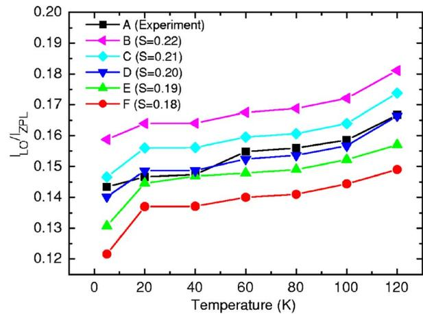
FIG. 3. (Color online) The measured and calculated intensity ratio of the first-order LO phonon sideband and the zero-phonon line (ZPL1) vs. temperature. Direct comparison of experiment with theory makes one to determine the Huang-Rhys factor  $S=0.20$ .
