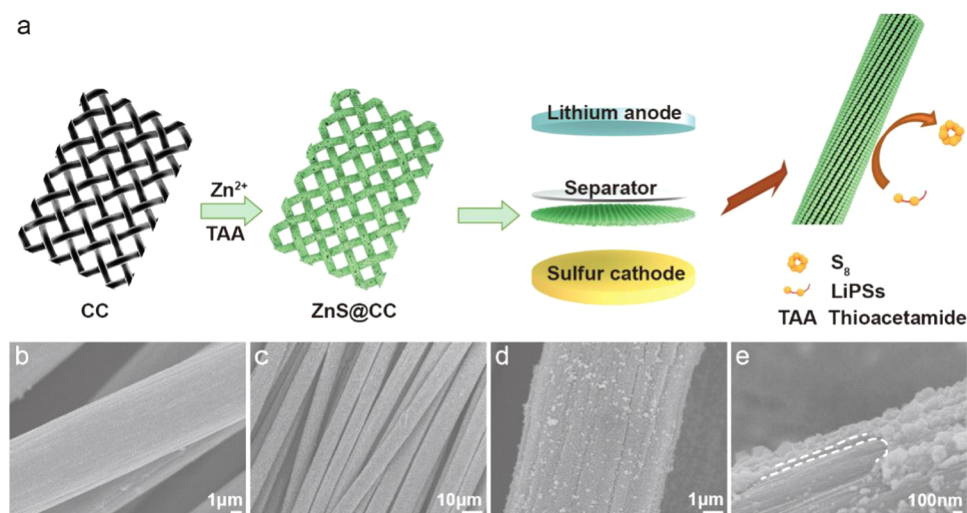
Figure 1. (a) Schematics of the fabrication process of ZnS@CC and the assembled cell model, (b) SEM image of treated CC, (c) and (d) low-magnification SEM images of ZnS@CC, and (e) high-magnification SEM image of ZnS@CC.
